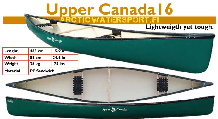
Incredibly versatile all rounder Upper Canada 16 is agile, stable and easy to handle canoe that allows you explore rivers and lakes. The boat keeps being very stable even when hitting bigger waves. The special grade 3-layer sandwich polyethylene construction makes it unsinkable canoe with very stiff and durable hull that weights only 36 kg. Capacity 320 kg.
