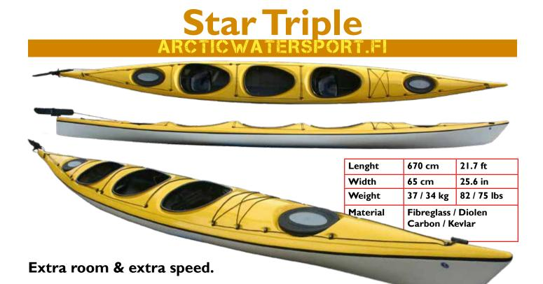
StarTriple is designed on the base of the test winner Star630. It is for paddlers who need extra room in middle cockpit for third person,pet or large gear. Long waterline and moderate rocker combined with well performing rudder gives great cruising speed and good maneuverability. This kayak is also ideally suited to paddlers with mixed abilities or families with young children that are seeking well performing and reliable kayak.
